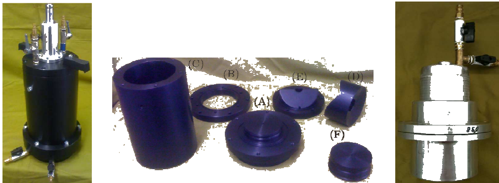
Figure 1: (left) Assembled aluminium cell with a load piston of diameter 2.5 cm, (middle) disassembled parts and (right) the load piston of diameter 10 cm for extension tests.
